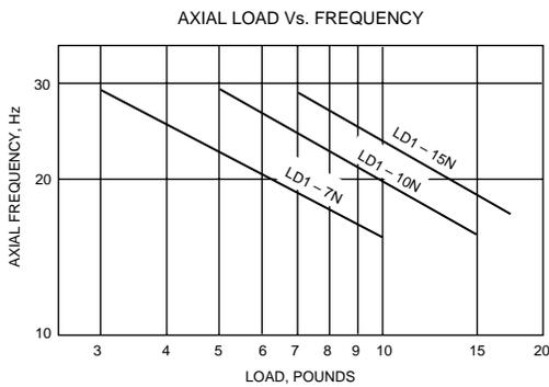
Tested with .036 in. D.A. input
