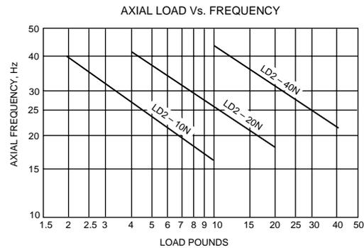
Tested with .036 in. D.A. input
