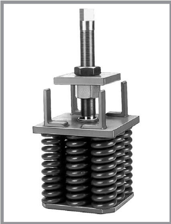
A heavy duty spring isolator most frequently used to support machines on deep concrete foundations such as forging hammers and roll grinders. The structural members cast through the foundation are supported by the UN isolator, and machine and foundation is levelled through adjustment of the isolator. Separate snubbing and damping controls are available. Load range to 35,000 lbs. per isolator and deflections to 1½" result in excellent shock and vibration attenuation.
